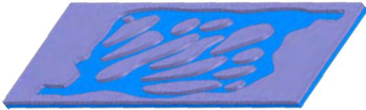
Figure 7. Conceptual design of a charge plate for industrial energy storage, with top interface layer removed. Inside are the topology-optimized flow channels, colored purple for Stellite® and blue for Inconel.
