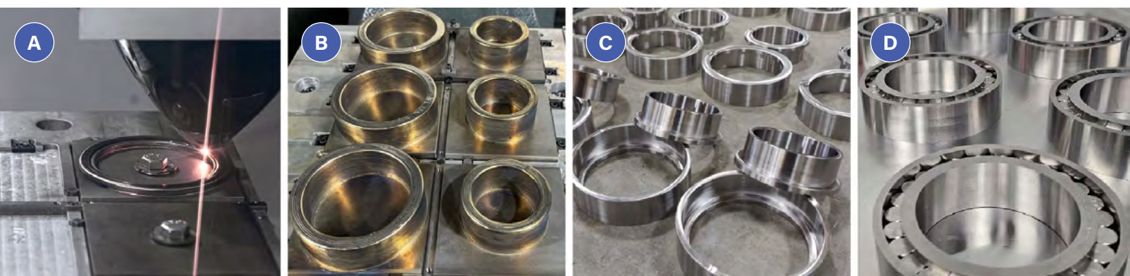
Figure 3. A superalloy bearing at different stages of the wire-laser hybrid process: (A) near-net build of ring; (B) rings after wire-laser DED; (C) inner and outer rings after CNC machining; (D) assembled bearings with rings and rollers.
