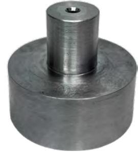
Figure 5. Multi-material sprue bushing produced using wire-laser hybrid manufacturing.
