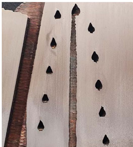
Fig.5.2.3: photo of a sectioned sample with teardrop-shaped cooling channels
