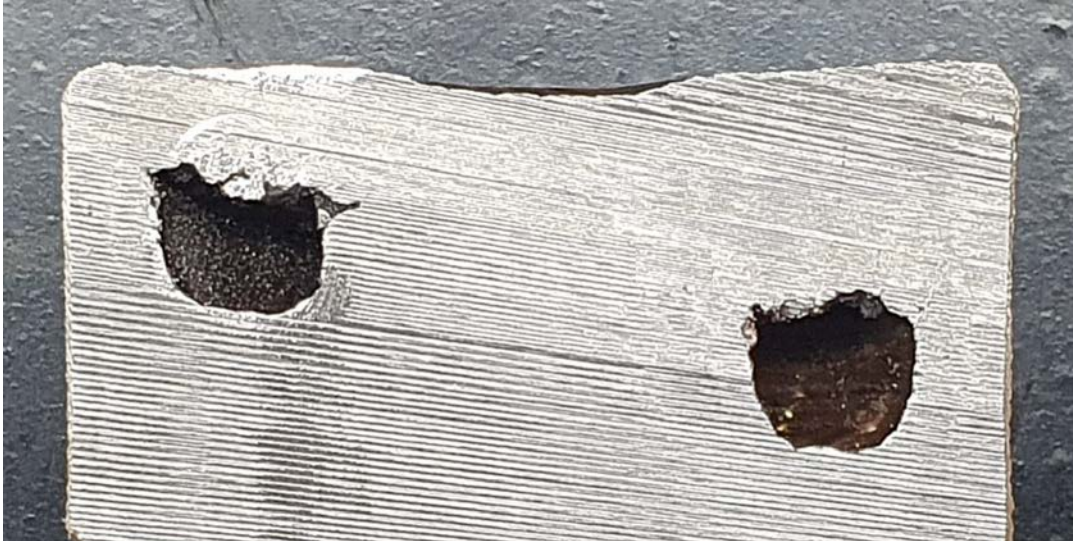
Fig.5.3.2: photo of a sectioned sample with square cooling channels
