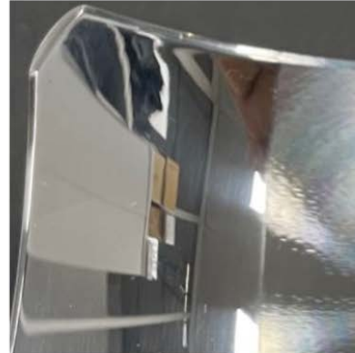
Fig. 4.3.2: Polishability of Tool Steel H11, index of high density.
