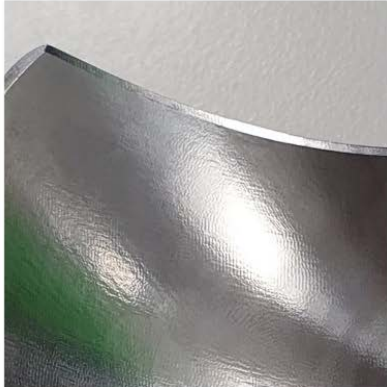
Fig. 4.3.2: Polishability of Tool Steel H11, index of high density.
