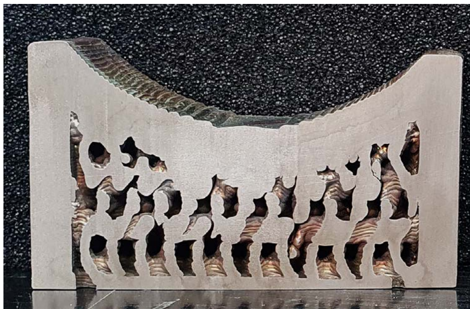
Fig.5.3.4: photo of a sectioned sample with gyroidal cooling channels
