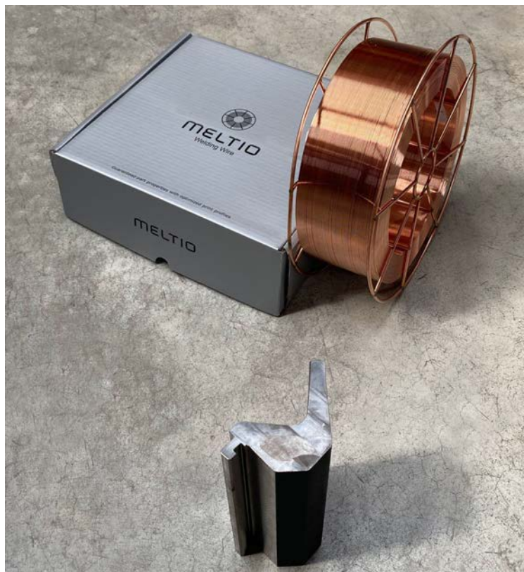
Fig. 4.3.1: Meltio Tool Steel H11 spool with sample part, a dual material Press Brake Tool with surfaces in Tool Steel H11 and core printed in Mild steel.
