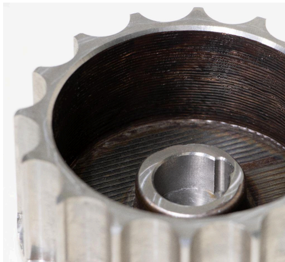
As-printed vs machined surfaces
