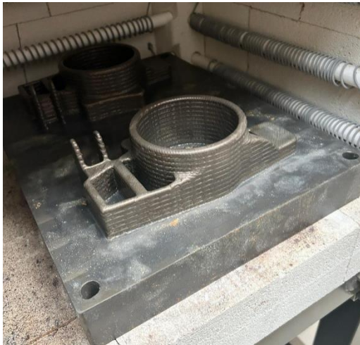
Figure 15. Rear Uprights after Heat Treatment.
