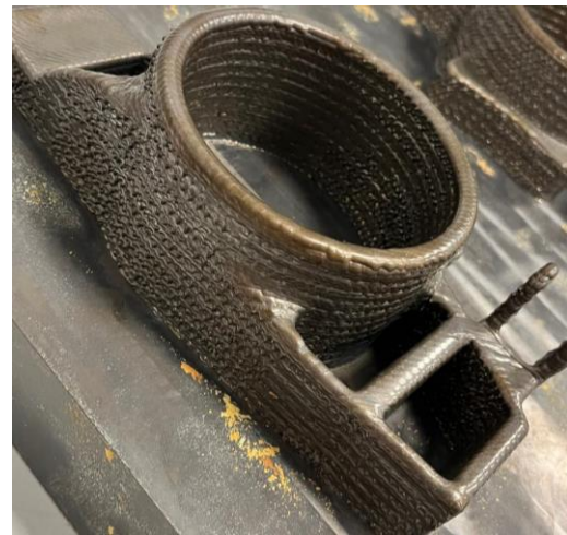
Figure 15. Rear Uprights after Heat Treatment.
