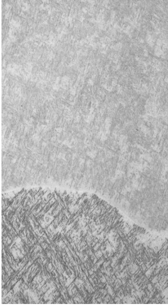
As-printed XY 100x Magnification
