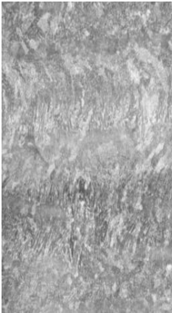
As-printed XY 100x Magnification
