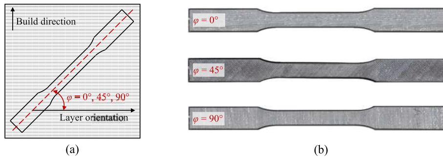
Fig. 4. Orientations of extracted tensile coupons: (a) angle definition, (b) typical coupons of different orientations.
