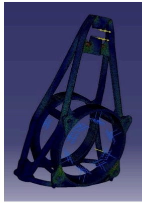
Figure 17: Lateral load case. Mesh size 0.5mm Figure 18: Lateral load stresses Figure 19: Lateral load displacements
