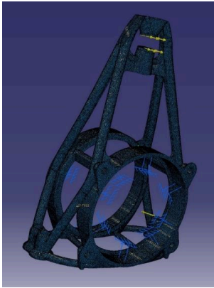
Figure 17: Lateral load case. Mesh size 0.5mm Figure 18: Lateral load stresses Figure 19: Lateral load displacements
