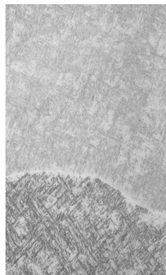
Gen II As-printed XY 100x Magnification
