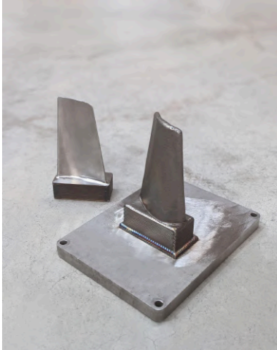
Comparison between turbine blade printed on the base and after removing and machining.
